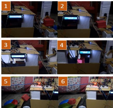
Figure 13. Color and weight sorting for Red color object
